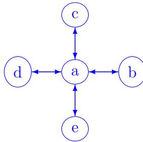
2. What is the average degree of the nodes in this network?  $(4 + 1 + 1 + 1 + 1 + 1(in) + 4 + 1 + 1 + 1 + 1(out))/5 = \frac{16}{5} = 3.2$  (give credit for 1.6 if #1 is undirected)
